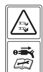
**Sharp blade(s). Beware of severing toes or fingers. Switch off and remove plug from mains before adjusting, cleaning or if the cable is entangled and before leaving the garden product unattended for any period. Keep the supply flexible cord away from the cutting blades.**
