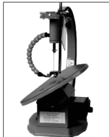
A bevel scale is provide under the work table as a convenient reference for setting the approximate table angel for bevel cutting.
