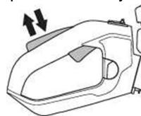
Check that the throttle trigger and throttle lockout move freely and that the return springs work properly.
