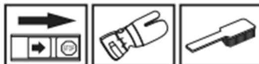
The filter oil contains a solvent to make it spread evenly through the filter. You should therefore avoid skin contact. Put the filter in a plastic bag and pour the filter oil over it. Knead the plastic bag to distribute the oil. Squeeze the excess oil out of the filter inside the plastic bag and pour off the excess before fitting the filter to the machine. Never use common engine oil. This would drain through the filter quite quickly and collect in the bottom.
