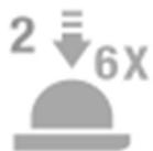
Press the air purge diaphragm repeatedly until fuel begins to fill the diaphragm (about 6 times). The diaphragm need not be completely filled.
