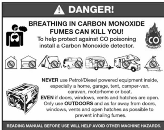
**DO NOT use in an enclosed area or moving vehicle**
