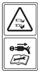
**Sharp blade(s). Beware of severing toes or fingers. Switch off and remove plug from mains before adjusting, cleaning or if the cable is entangled and before leaving the garden product unattended for any period. Keep the supply flexible cord away**
