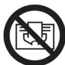
**Make sure that the air inlet and outlet openings are not blocked. To avoid any risk of fire, do not cover the heater (ex. With clothes)**
