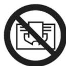
**Make sure that the air inlet and outlet openings are not blocked. To avoid any risk of fire, do not cover the heater (ex.**
