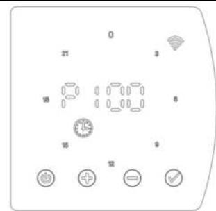
Tap for 3s to modify P1-P7 programming, tap keys to adjust, stepping by 1H. Press to run comfort mode displaying , press to run Eco mode, displaying
