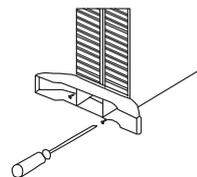
Before using the heater, the feet (supplied separately in the carton), must be fitted to the unit. These are to be attached to the base of the heater using the 4 self-tapping screws provided, taking care to ensure that they are located correctly in the bottom ends of the heater side moulding
